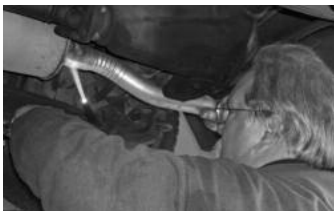
IN THE BELLY OF THE VOLVO. Eric Bjorklund is a study in focus as the welds a muffler.
