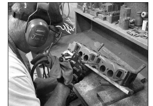
Jim from Huffaker Engineering modifying the cylinder head for Bruce's P1800.
